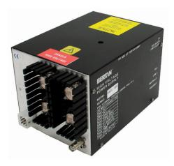
Spellman's Bertan brand of 603C modular high voltage power supplies offer well regulated, fixed polarity outputs up to 30kV, that operate off a standard switch selectable 115/230Vac input. These fully enclosed modules are designed for bench top or OEM applications like spectrometers, detectors, imaging and electron beam usage.
